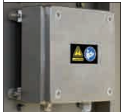
FIM enclosure box mounted onto the conveyor
